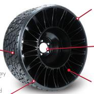
Zero-degree belts and ComposiCoil™ proprietary design provide great lateral stiffness, while resisting damage and absorbing impacts.
