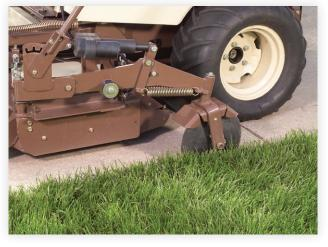
Left (trim side) mount for side- and rear-discharge decks.
