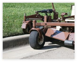
A reversible, concave, self-sharpening, tempered blade and weighted hub assembly maintain a clean, sharp edge from sidewalk, curb or turf.
