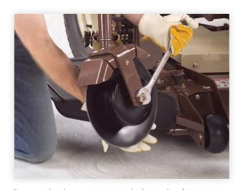
Reverse disc by removing one bolt to edge from the turf.
