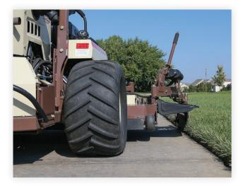
Edge-EZE™ discharge shield allows you to blow debris off sidewalk into turf.
