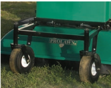
FRONT-MOUNTED CASTER WHEELS and independently floating spray chambers follow ground contours for precise and even spray application.
