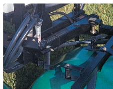
BREAKAWAY WINGS protect the sprayer and small trees from damage caused by accidental contact.
