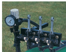
EASY REACH TeeJet® valves, pressure regulator and pressure gauge are all within reach and sight of the operator.
