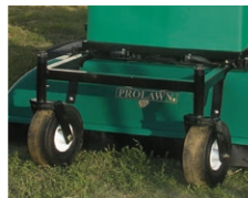
FRONT-MOUNTED CASTER WHEELS and independently floating spray chambers follow ground contours for precise and even spray application.
